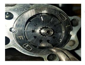
Remove c-clip on the shaft and use needle nose pliers to remove impeller vanes. Reinstall back cover, torque to 23-31 ft-lbs. Install plug with copper washer and torque to 36-51 ft-lbs.
