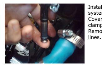
Install metal plug onto barb for return hose of Hicas system on the power steering reservoir.
