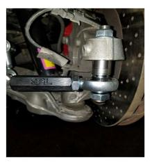
The following pictures show possible bumpsteer adjustment settings, using various combinations of spacers. The stock tie rod end corresponds to the 3<sup>rd</sup> setting (with two adjustment spacers and no misalignment spacer).
