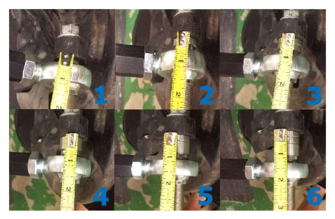
For most installations on stock knuckles, we recommend using **4th setting**.
