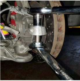
Remove the two 5/8"-18 Jam Nuts, and install the Spacers (3, 4, 5). Install the locking nut on bottom (9). This nut will take some effort to thread (about 20 ft-lbs. of torque) as it is a metal, crimping/locking nut. Torque to 80 **ft-lbs**.
