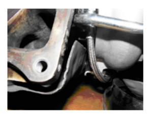
For new turbo installation, pre-assemble the upper oil line assy to the turbo as in the pic below:
