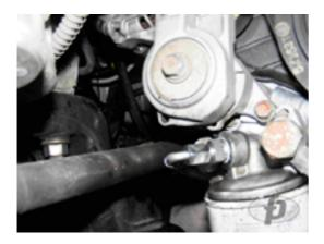
This plug is damn near impossible to remove without breaking the loctite bond by heating to over 400F.
