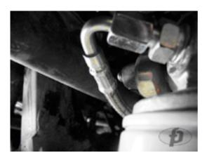
Route hose along factory oil cooler lines, attach with zip ties. Make sure hose is kept away from the spinning bits such as the A/C pulley, extra zip ties are provided if you are nervous.
