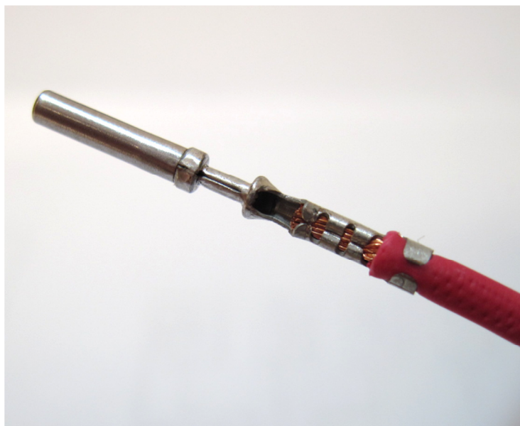
Image shows a properly crimped terminal. Top View.
