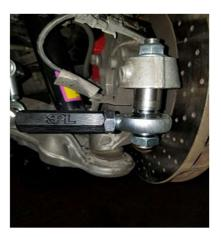
The following pictures show possible bumpsteer adjustment settings, using various combinations of spacers. The stock tie rod end corresponds to the 3<sup>rd</sup> setting (with two adjustment spacers and no misalignment spacer).
