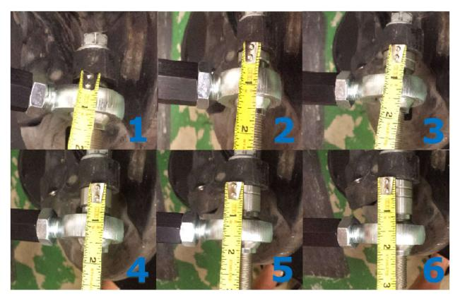
For most installations on stock knuckles, we recommend using **4th setting** (one ½" spacer, no ¼" spacers).
