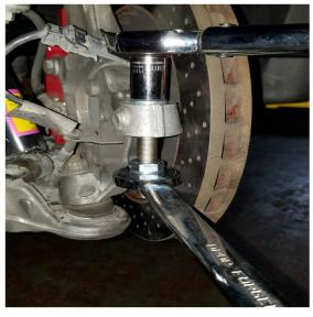
Remove the two 5/8"-18 Jam Nuts, and install the Spacers (3, 4). As pictured on left, the Tie Rod Ends are installed with one ¼" spacer (3) and one ½" spacer (4). Install the locking nut on bottom (8). This nut will take some effort to thread (about 20 ft-lbs. of torque) as it is a metal, crimping/locking nut. Torque to 80 **ft-lbs**.
