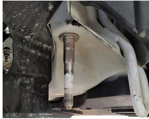
6. Install the SPL Parts Control Arm at subframe end first. The large Offset Spacer should go to the rear of the car, and the small offset spacer to the front of the car on the joint. Place the bolts through, but do not tighten yet as this will make it more difficult to finish the installation.
