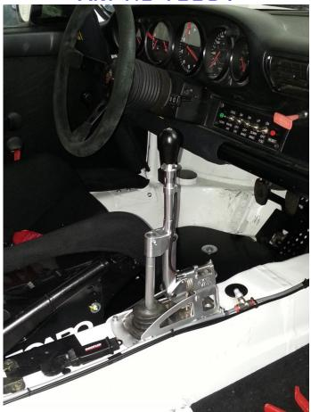
The CAE shifter is designed for Porsche's cars without interior equipment. If center console is mounted, it must be removed or modified to achieve an acceptable space for the shifter.
