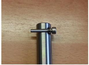
Tighten the screw lightly and fix it with the wire.
