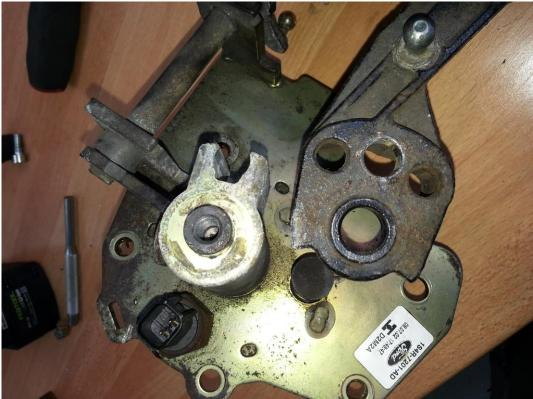
To do this, first drill out the rivet (red circle) (dia 12mm), then loosen the Torx screw and pull the lever off the selector shaft Install the CAE shifter and tighten with the original Torx screw.
