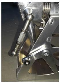
Pull off the side tie rod on the shifter from one of the balls
