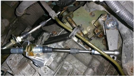
Mount the sealing collar on the selector lever ball head, grease the ball heads well
