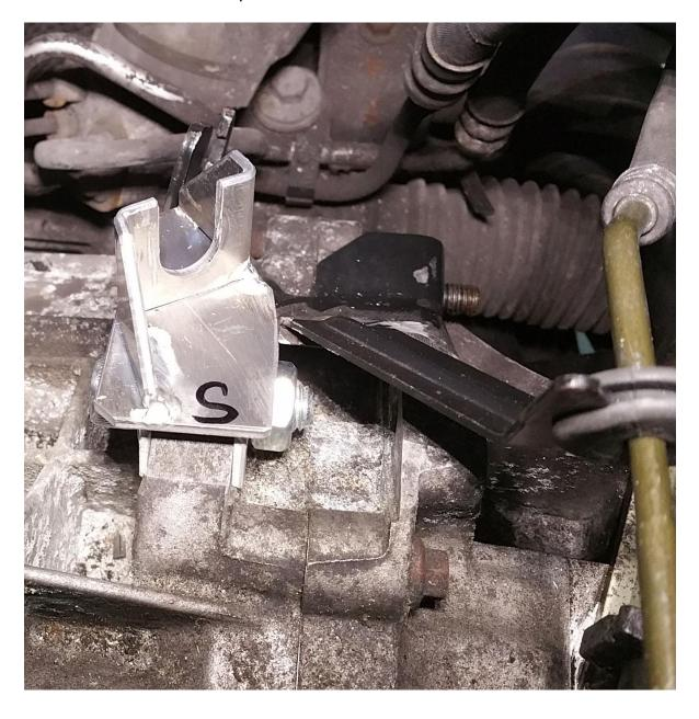
The original gear shifter must be removed from the stem:
