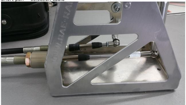
**Shiftcable (S) L=1200mm** - long ball cups and long M6 threaded with bronze extension sleeve -
