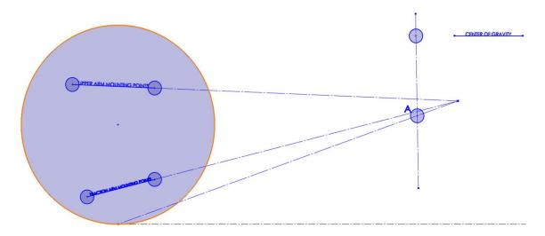
The following diagram shows what happens when you raise the subframe closer to the chassis. For this example, we are comparing what happens to the anti-squat when the ride height remains the same. When the subframe is raised, the rear "instant center" is raised as well, that moves point A up and increases anti-squat.
