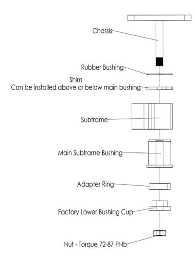
Remove subframe and OEM subframe bushings. The OEM subframe bushings can either be pressed out or cut out. The entire OEM bushing must be removed, including all the outer metal "shells" (race). When the OEM bushing is completely removed, there should just be 1 ring of steel left that is part of the subframe itself. Press in the main bushing from the bottom of the subframe.
