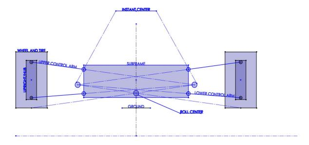
The following diagram shows the subframe raised closer towards the chassis (no more gap between subframe and chassis), and the ride height lowered the same amount. The roll center position is un-changed.
