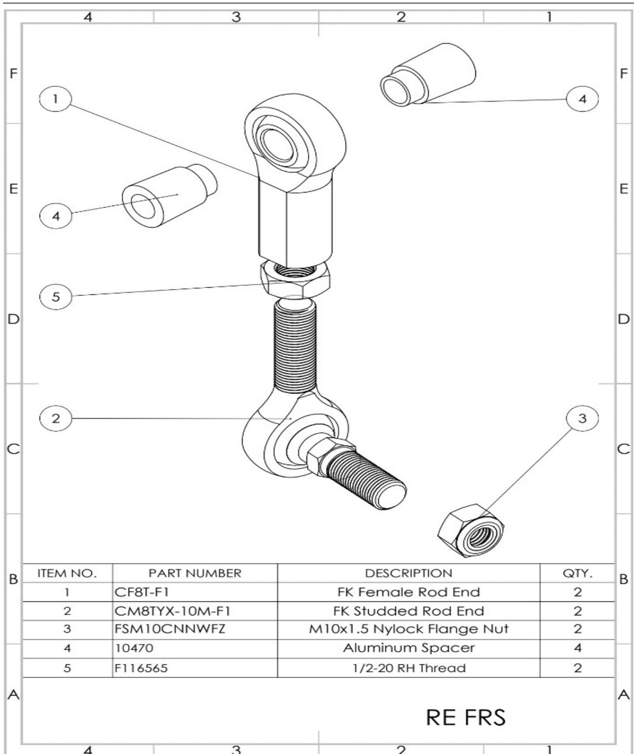
Torque the Flange Nuts (3) attaching the endlinks to the sway bar to 15-20 **ft.-lbs. DO NOT OVERTORQUE!**
