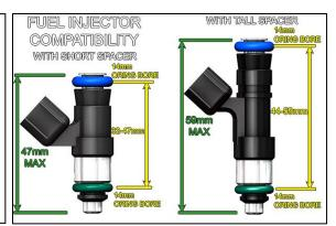
6. Insert the small end of the phenolic mounting spacer into the fuel rail mounting boss, as shown. Secure the fuel rail onto the intake manifold, ensuring all injectors seat properly.
