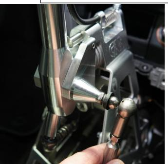
Turn the right (long) coupling rod to the Llever by turning it so that the ball socket can be pressed on without length change.
