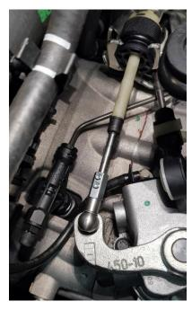
For better shift feeling we also recommend to remov the absorber weights on the gear lever, this is not mandatory for the function
