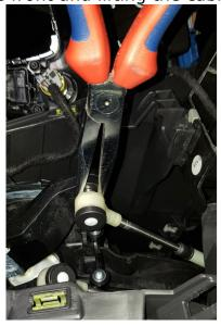
remove the original shift lever (4 screws)
