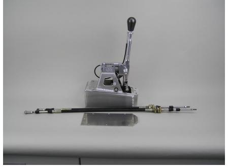
The shifter is intended for racing cars without interior equipment. If center console is mounted, it must be dismounted or modified to achieve an acceptable space for the cables. The new unit should be mounted directly on to the floorboard, so part of the carpet must be removed.
