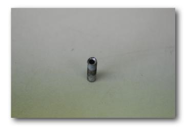
5. The next job is to assemble the new master cylinder and bracket. It is necessary to remove the standard studs from the clutch cylinder and use the cap head bolts provided.
