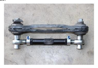
3. Install the SPL Parts Arm using the OEM hardware. Please ensure the Tapered Spacer (9) provided mates up with the tapered section of the knuckle. Tighten the bolts at the subframe to 74 **ft.-lbs.** and the bolts at the knuckle to 135 **ft.-lbs**. **DO NOT OVERTORQUE!** SPL Parts is not liable for any issues due to overtorque.
