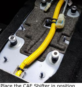
Place the CAE Shifter in position and insert the shift cables into the shifter housing; Immediately insert the cables into the respective bracket
