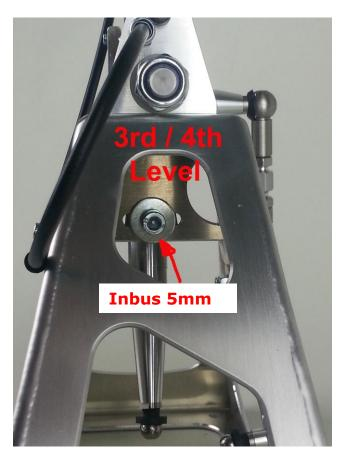
This is the basic setting of the shifter and must be carried out correctly !!
