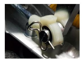
Generally grease each ball socket and bearing pin & bushings.
