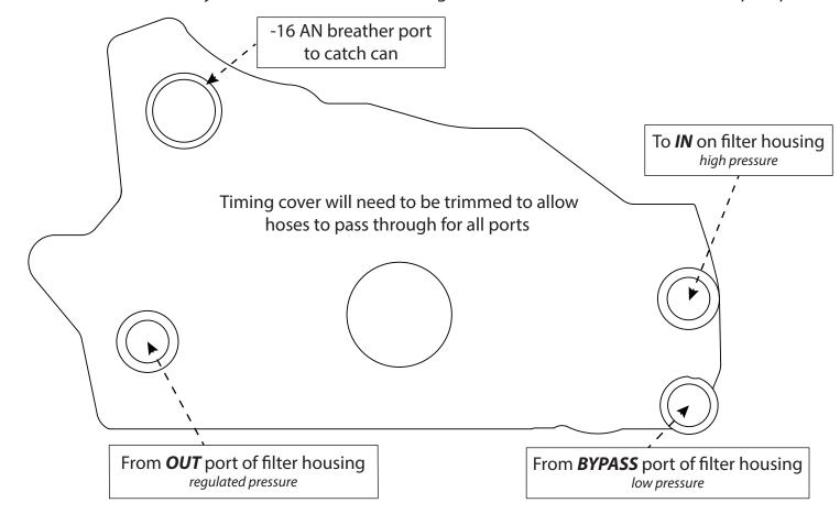
**CAUTION** Oil pressure regulator is not set. Oil pressure will need to be monitored and adjusted accordingly.
