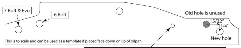
Avoid placing too much RTV near this hole. It needs to be able to relieve pressure from front of pump to operate correctly.
