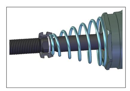
of the Spring Retainer. The Wire Lock Ring should register against the taper of the groove past the wrench flats.
