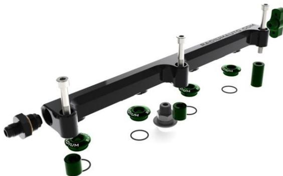
7. As a test, push the fuel injectors downward until they bottom out. Now inspect the injectors' upper O-rings and confirm they are still inserted into the fuel rail injector bores. Do not pressurize the fuel system until the proper height is achieved.
