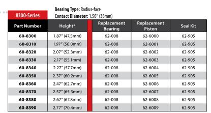
\*Height can be reduced by .050" (1.27mm) by removing the shim that is located under bearing within the piston
