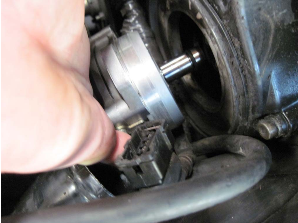
Figure 43: Reinstalling the CAS sensor
