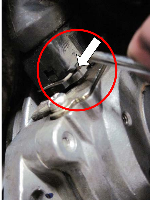
Figure 9: Pry here to remove this clip
