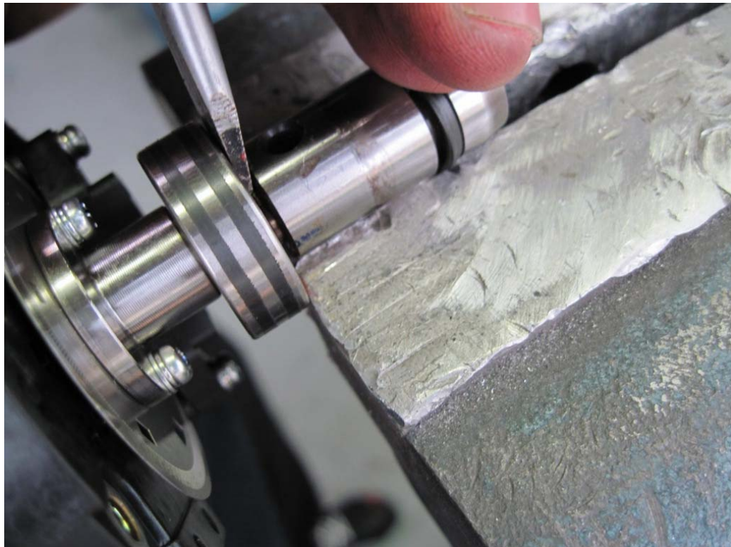
Figure 26: Removal of star socket using 1/4" flat screwdriver
