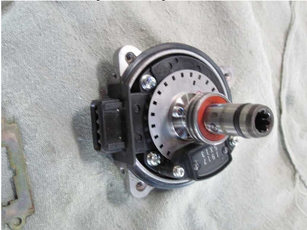
Figure 40: CAS rubber seal reinstalled
