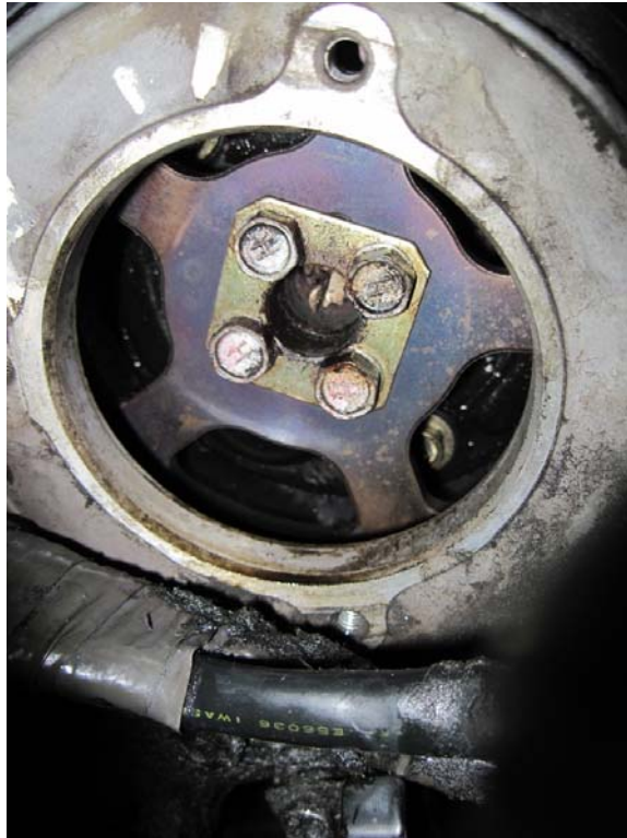
Figure 13: CAS sensor removed
