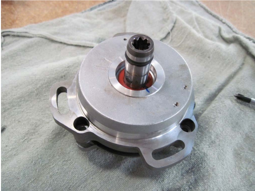
Figure 41: Housing cover reinstalled
