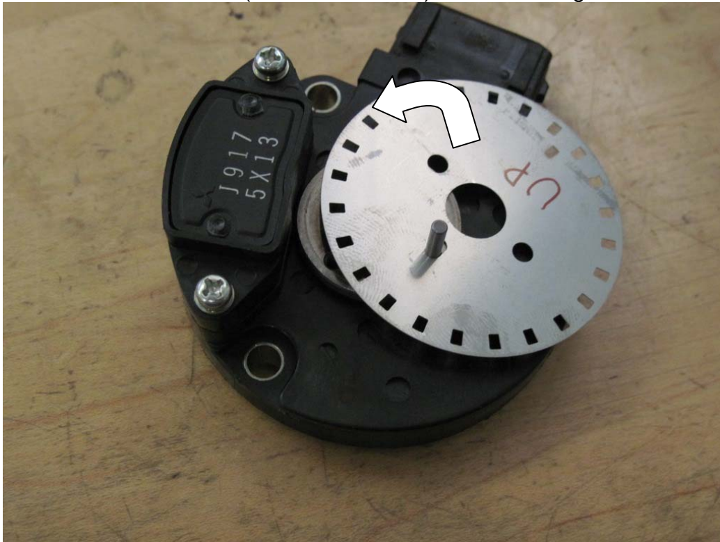
Figure 33: AEM trigger disc being installed
