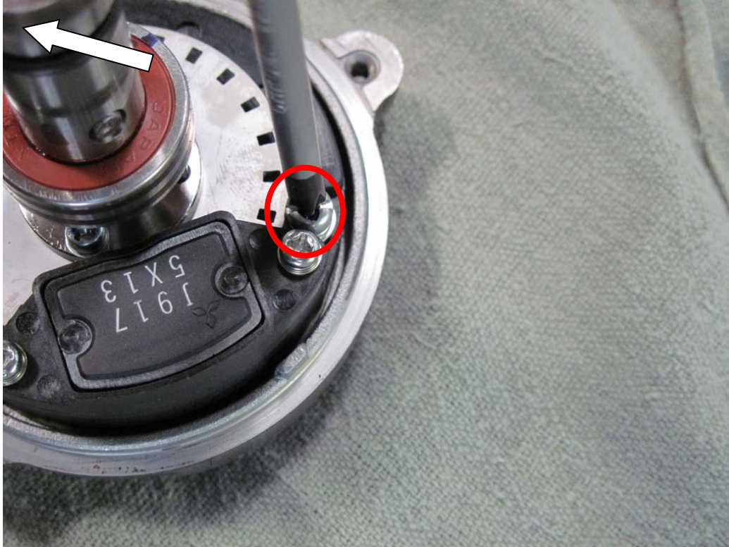
Figure 39: Reinstallation of CAS sensor screws
