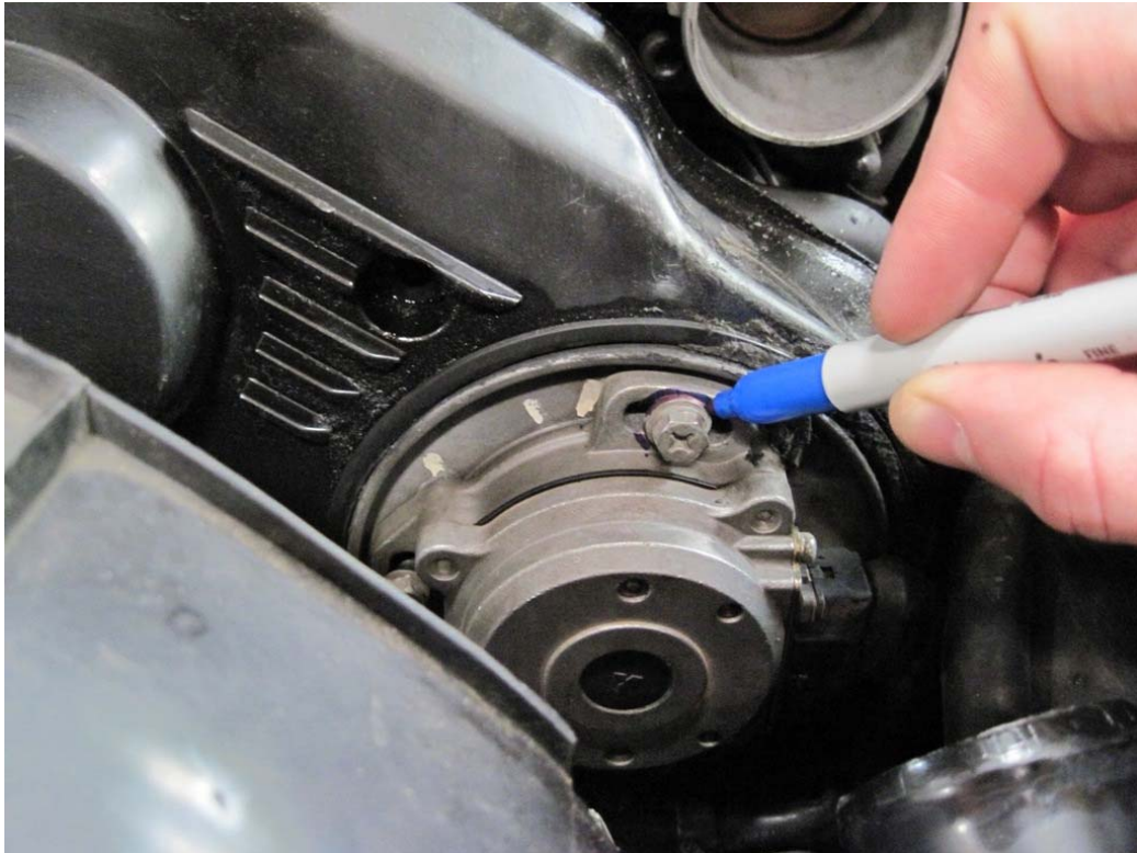
Figure 7: Marking position of CAS sensor
