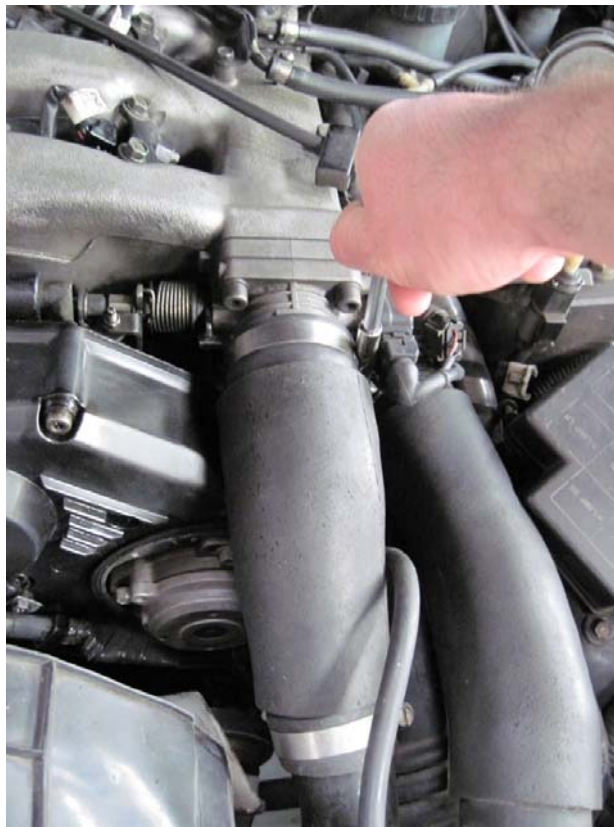
Figure 5: Removal of intake tube using 8mm socket
