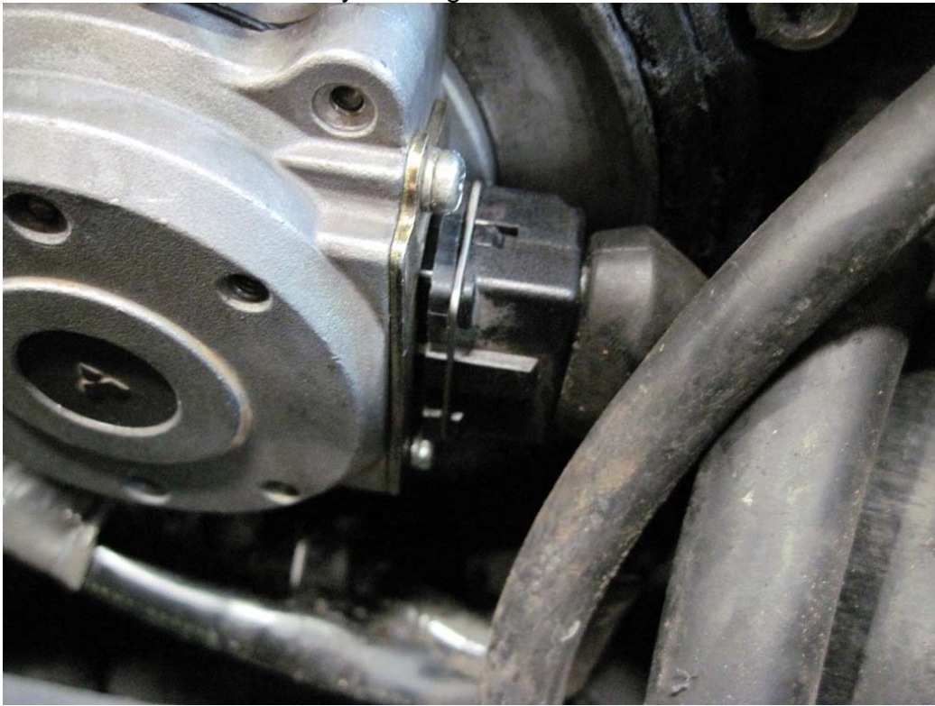
Figure 45: Replacing CAS sensor connector
