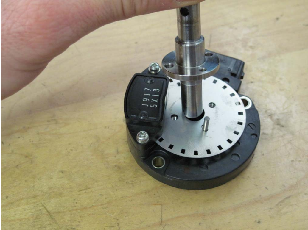
Figure 34: CAS sensor shaft reinstallation
