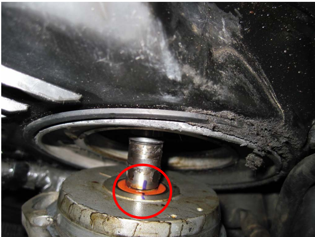
Figure 12: Mark shaft relative to housing for correct reinstallation onto cam
