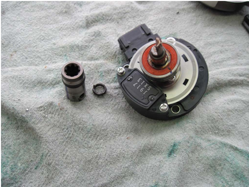
Figure 27: Star socket removed from CAS sensor
