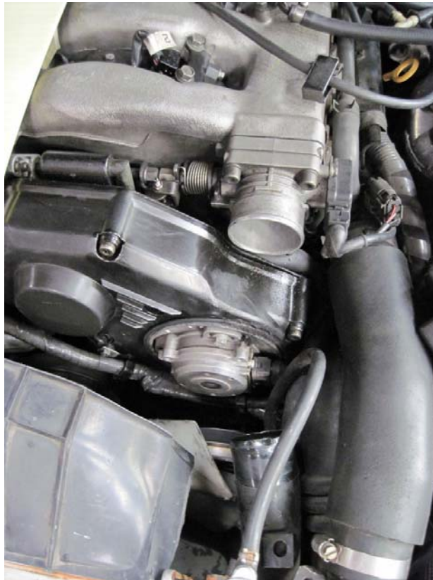
Figure 6: Intake tube removed to access CAS sensor
