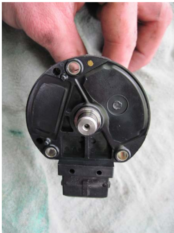
Figure 24: CAS sensor removed from housing
