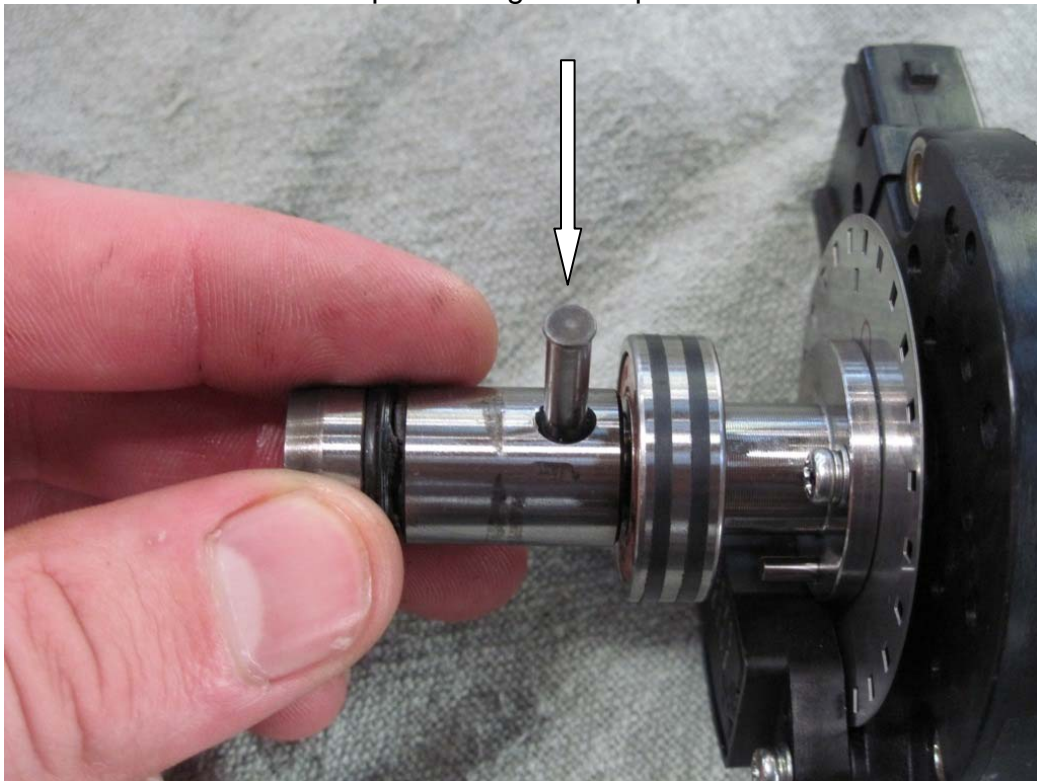
Figure 38: Aligning the star socket retaining pin
