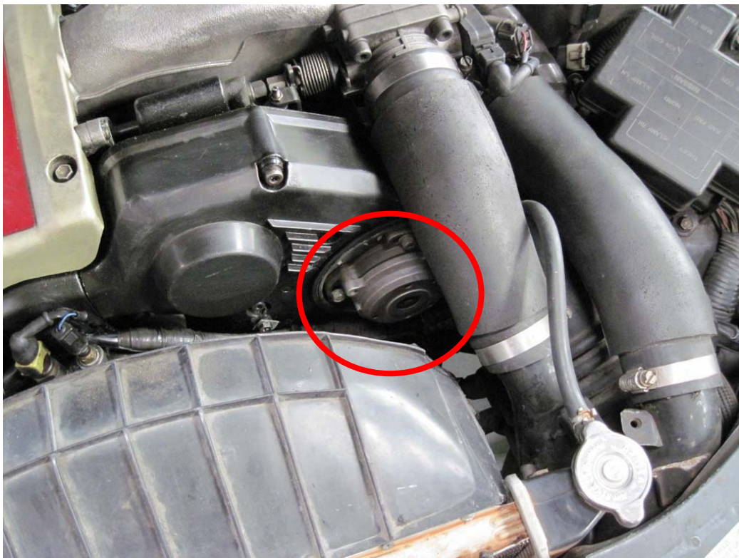
Figure 2: Location of the CAS sensor
