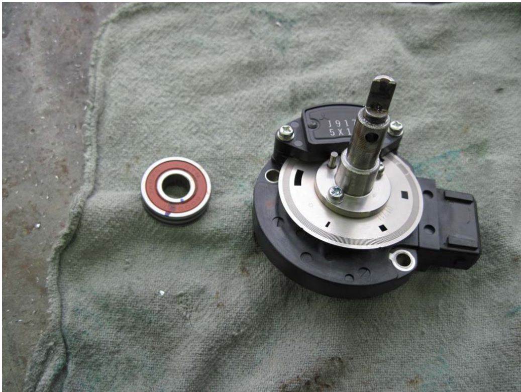
Figure 29: Bearing removed from shaft
