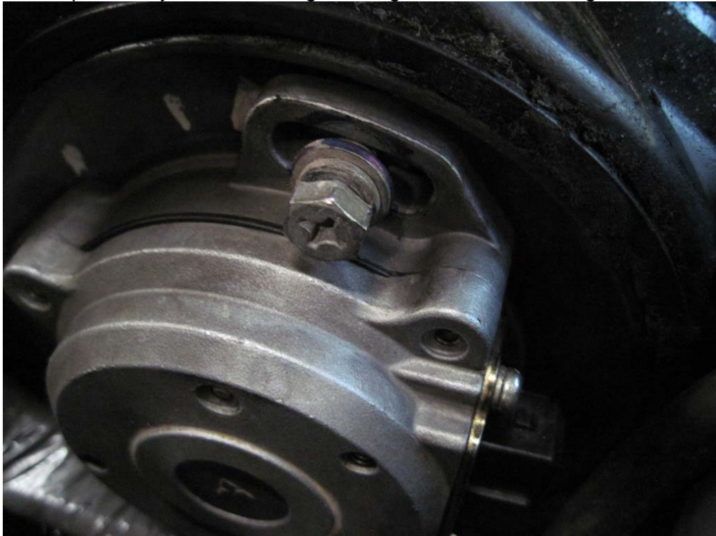
Figure 44: Reinstalling CAS sensor bolts
