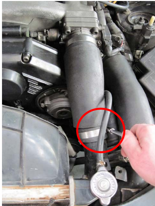
Figure 4: Removal of intake tube using 8mm socket
