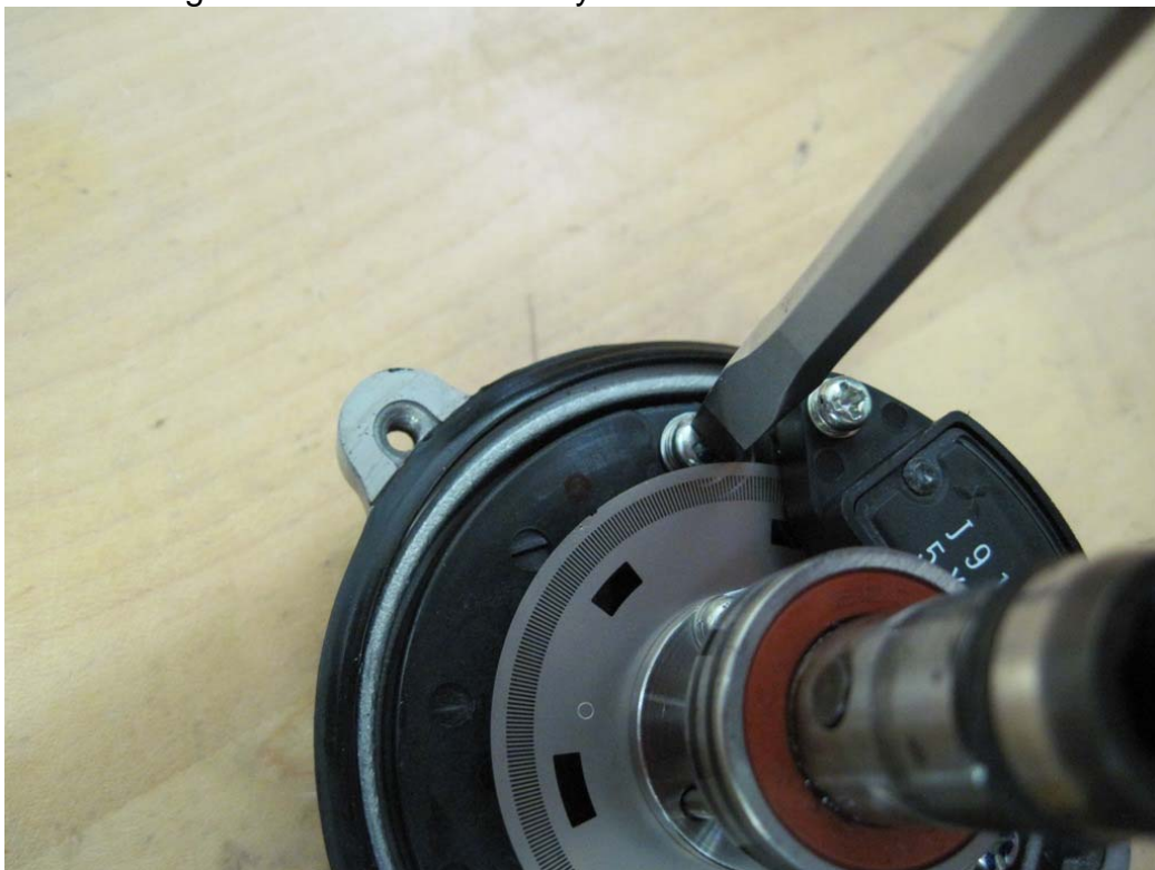
Figure 18: Remove 3 screws holding sensor using 1/4" flat screwdriver
