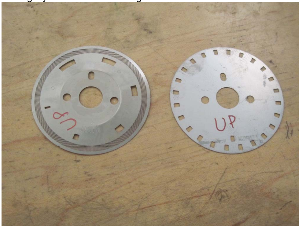
Figure 32: Comparison of original and AEM trigger discs
