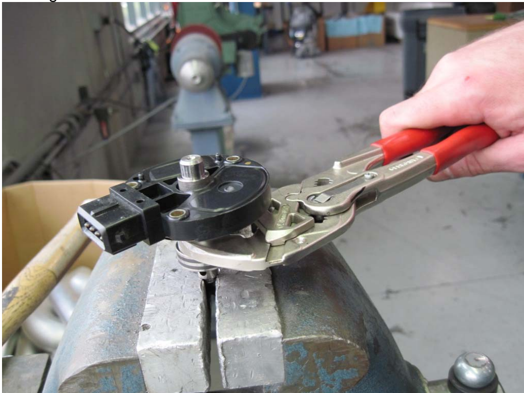
Figure 28: Removal of bearing from shaft using pliers
