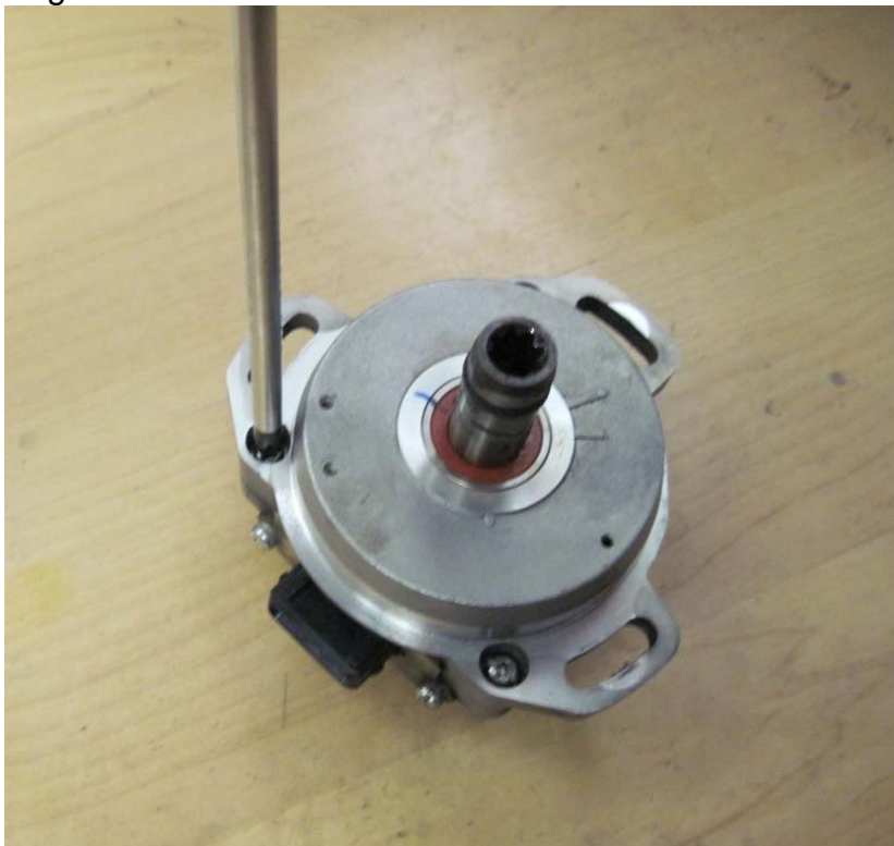
Figure 14: Taking apart CAS assembly using number 2 Phillips screwdriver
