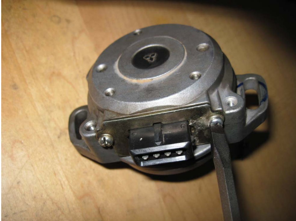
Figure 15: Removing seal cover on CAS assembly using ¼" screwdriver
