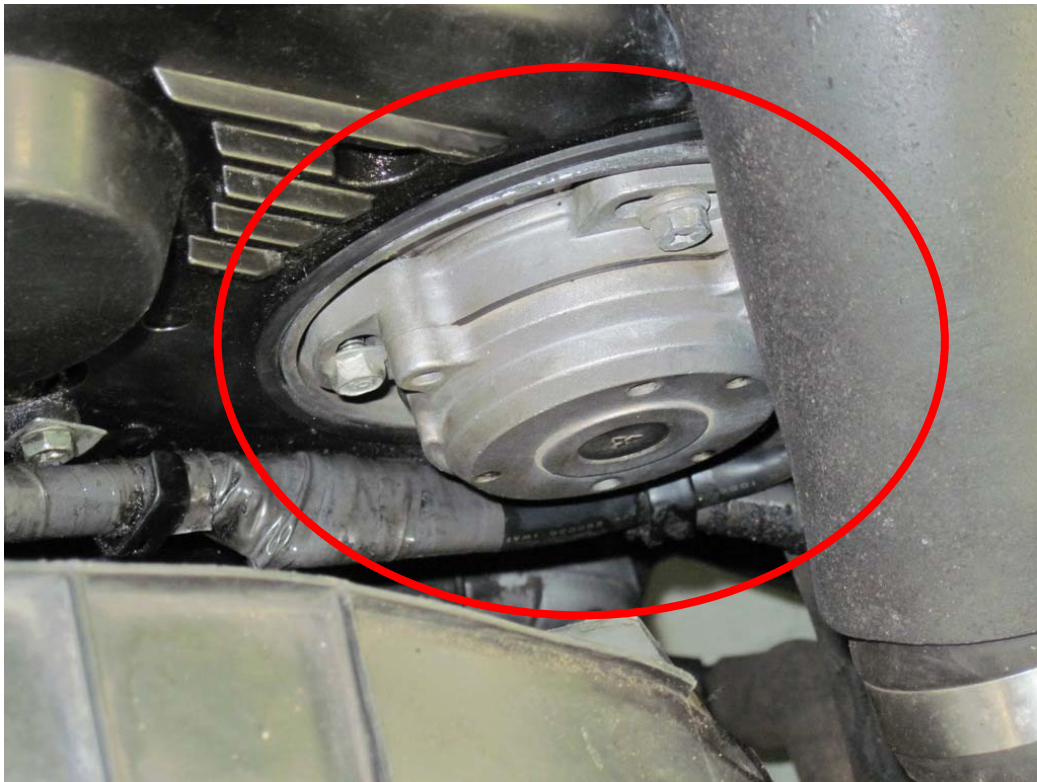
Figure 3: Close-up of CAS sensor
