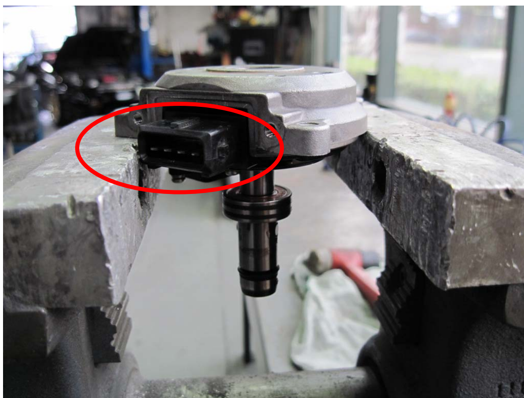
Figure 22: Mounting CAS assembly in vise to separate from shaft
