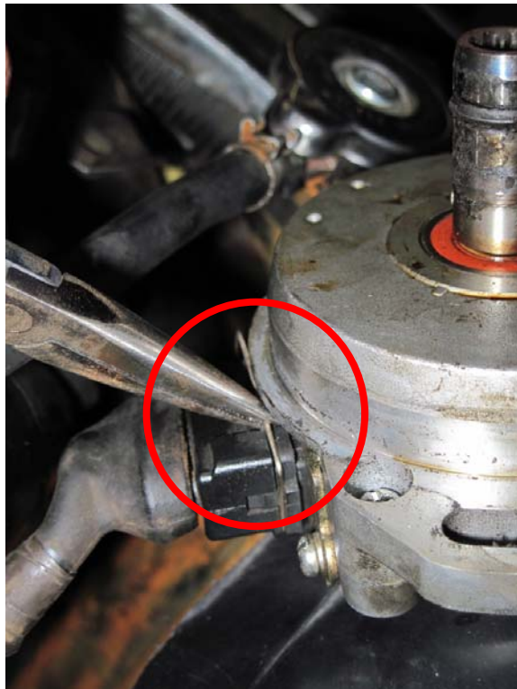
Figure 10: Remove clip with needle-nose pliers
