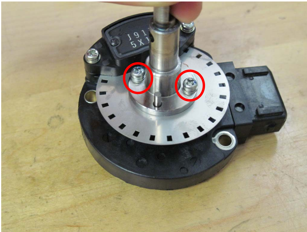
Figure 35: Screws for CAS shaft replaced
