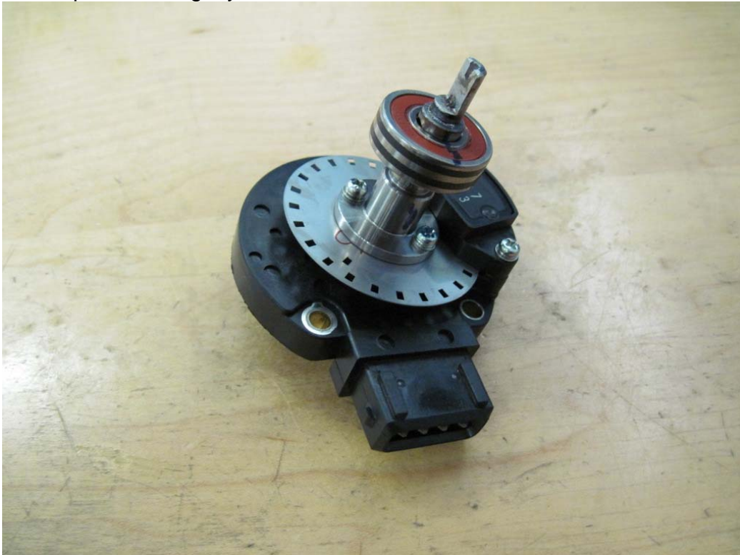
Figure 36: Bearing placement on CAS shaft
