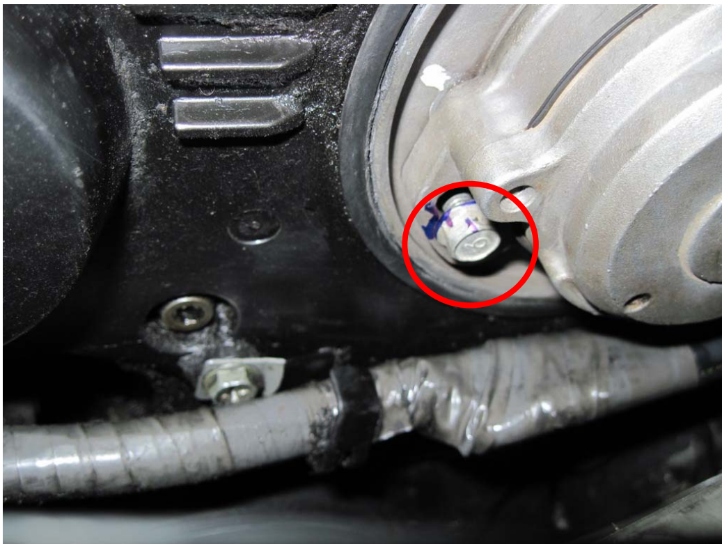
Figure 8: Marking position of CAS sensor
