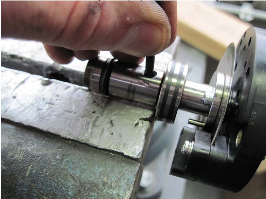
Figure 25: Removal of pin using 1/8" pin punch
