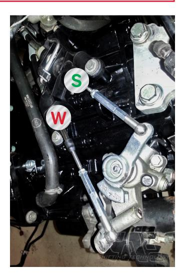
(i) PLEASE NOTE: ! Check cables for "end position free travel". When a gear is engaged, there must still be a residual travel available on the rope! (Picture A, B, C)
