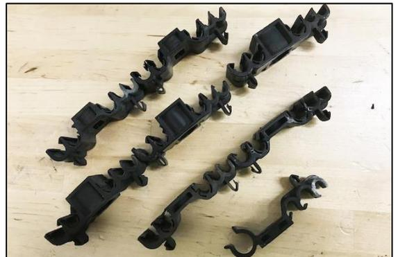
9. Using the OEM hardware and a 10mm socket wrench, install the 4 Radium retainers.
