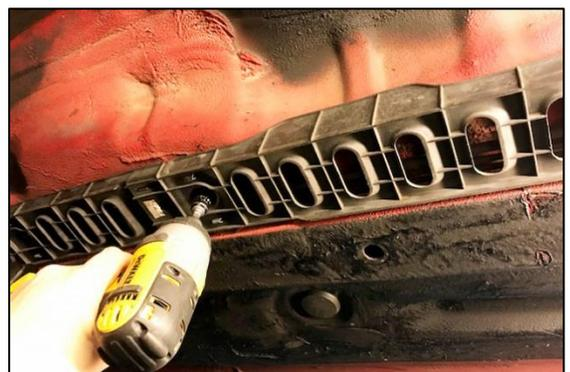
4. Pry the locking tabs to release the plastic hard line covers.
