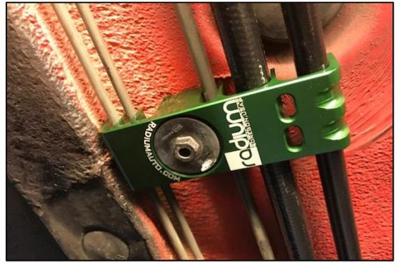
10. Using the provided cable zip ties, secure the innermost line to the retainers, as shown.
