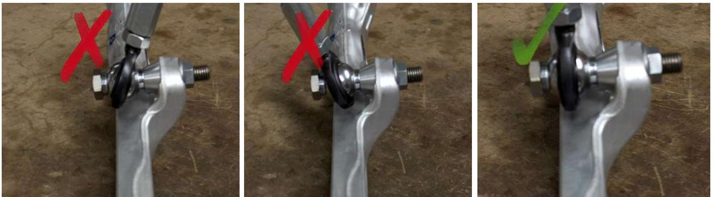
As a rule, you want the endlink to be as close to vertical as possible. If the bearing is not installed with sufficient articulation angle, then under suspension travel, the endlink will bind. To obtain good articulation, use the extra ring spacers supplied to adjust the position of the ball joint at the lower arm to best match the alignment to the installation hole on the sway bar:
