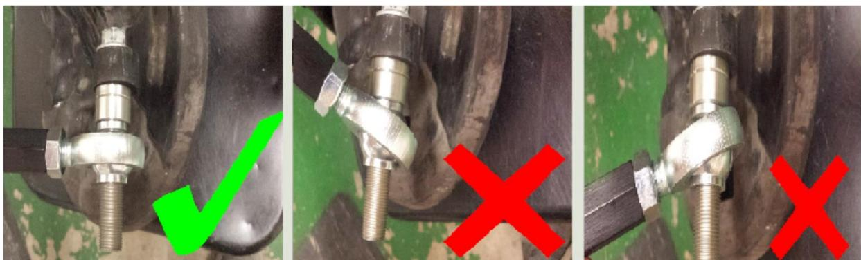
Note that the inner tie rod end can rotate freely, so the picture on left is not binding even though the edge of the ball is touching the housing. If uncertain, try rotating the inner tie rod by using a wrench on the hex part of the inner tie rod. To do this, tighten down the two jam nuts that go against the hex buckle of the outer tie rod end. Any excess thread below the bottom nut can be trimmed or cut off as needed (e.g. for wheel or steering bump stop clearance).
