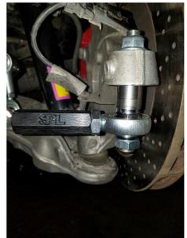
For most bumpsteer applications, it is a good rule of thumb to try and get the tie rod end as close to parallel to the lower control arm as possible. Verify there are no clearance issues with the knuckle, subframe, or other suspension arms before putting the car back on the ground.
