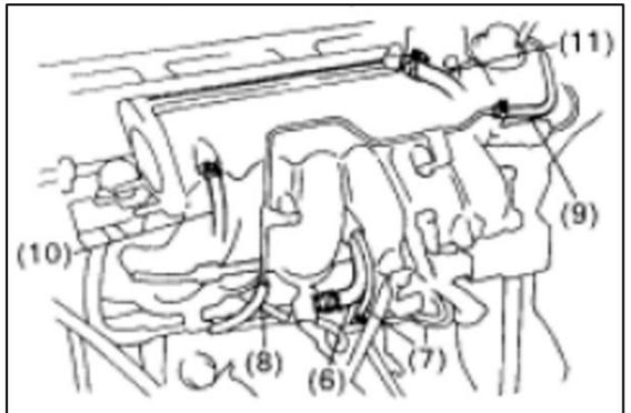
3. Disconnect EGR gas temperature sensor connector.
