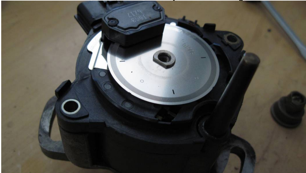
Figure 5: Original CAS screw and collar removed
