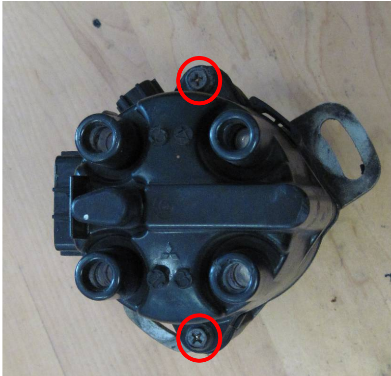
Figure 1: Distributor cap removal
