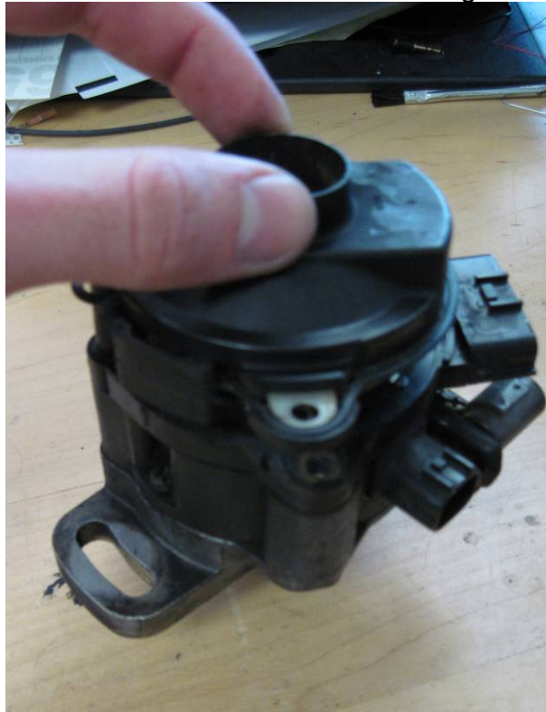
Figure 3: Removal of internal cover over CAS disc
