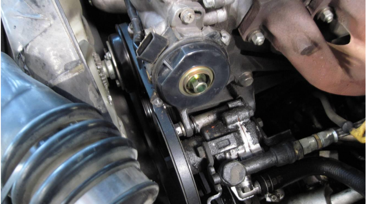
Figure 13: Internal plastic cover reinstalled
