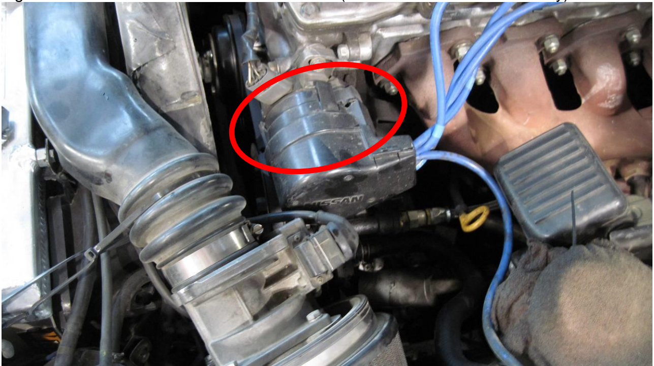
Figure 2: Location of CAS sensor (underneath distributor cap)
