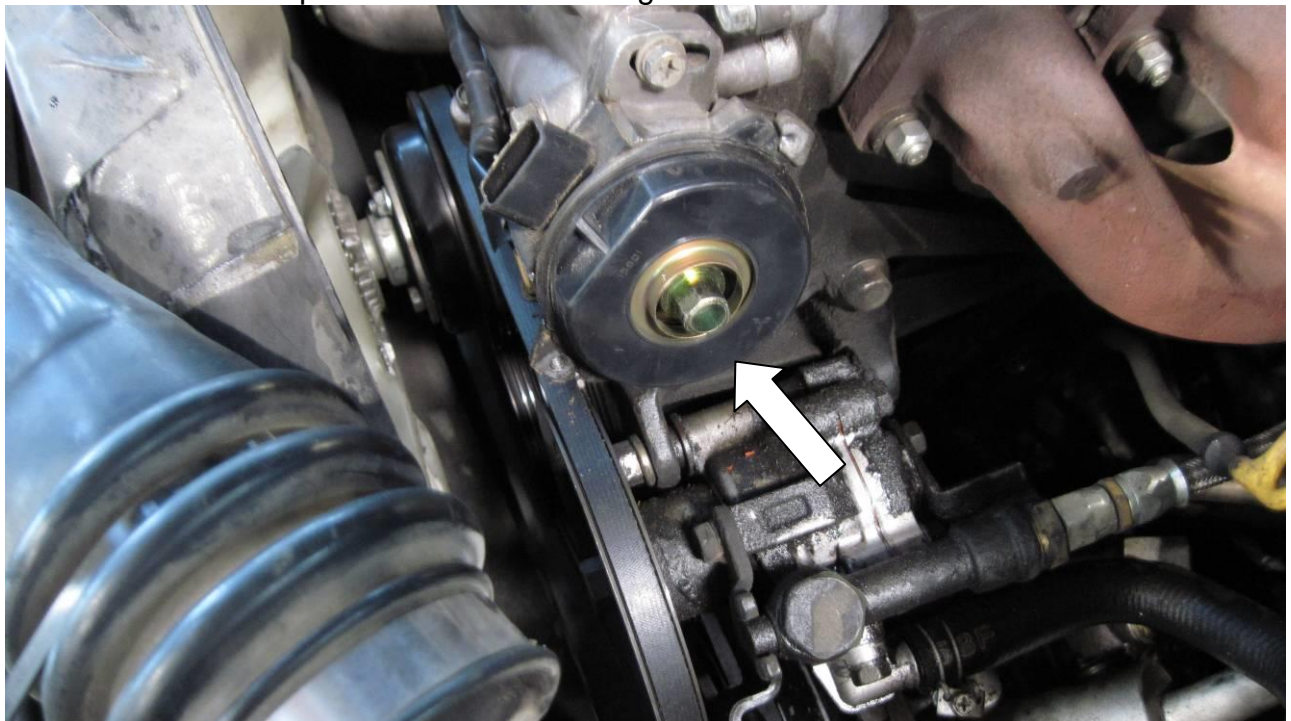
Figure 6: Internal plastic cover to be removed
