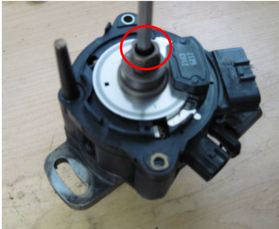
Figure 4: Removal of screw holding on CAS disc
