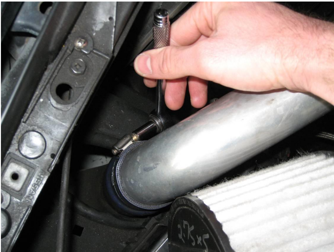
Figure 5: Removal of intake tube
