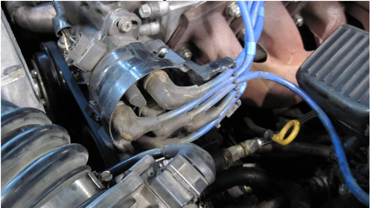
Figure 3: Plastic wire cover removed
