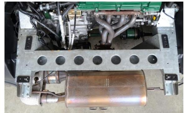
J. Line up the larger hole in the shims with the threaded holes in frame. Make a mark on the frame at the smaller countersink shim holes with pen. Repeat this process at all four locations.
